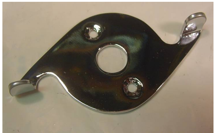
Right: reproduction bandchange lever made by Pat Jones, VE7PRJ, using another S.640's lever as a prototype. A piece of scrap mild steel, lots of Pat's elbow grease/skill and a local chrome-plating company did an excellent job!
