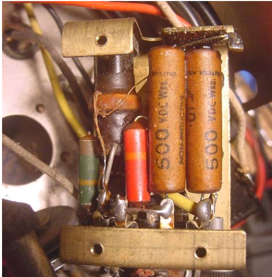
Above: BFO unit – before and after replacing the wax-paper capacitors and resistors
