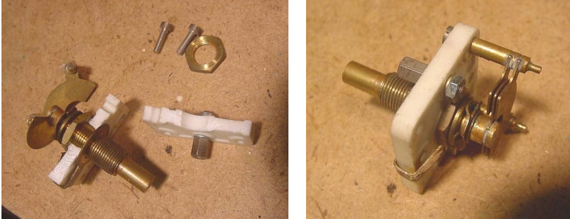
Above: BFO capacitor repair – careful cleaning, a few drops of super-glue, and two 6BA-tapped spacers carefully cut to the correct length and its as good as new
