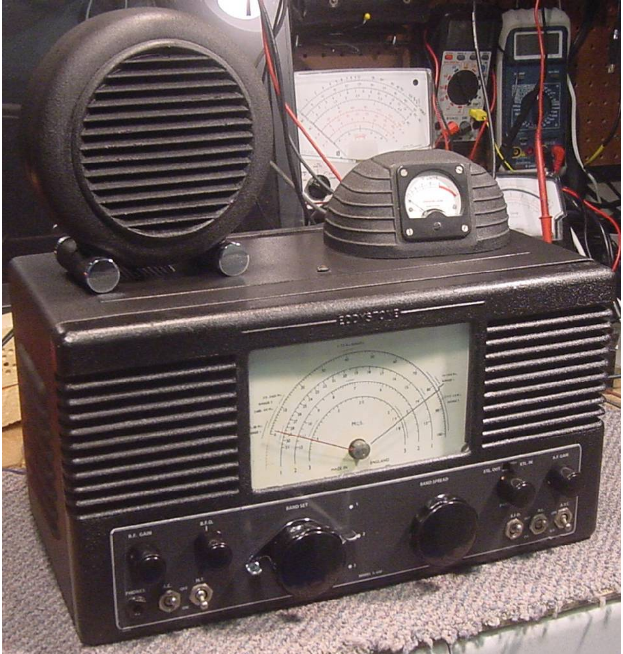
Above: Restored S.640 with matching 7" loudspeaker (Model 688) and Signal Strength Meter (Model 669). Below: serial number stamped on the IF/1 st AF sub-chassis.
