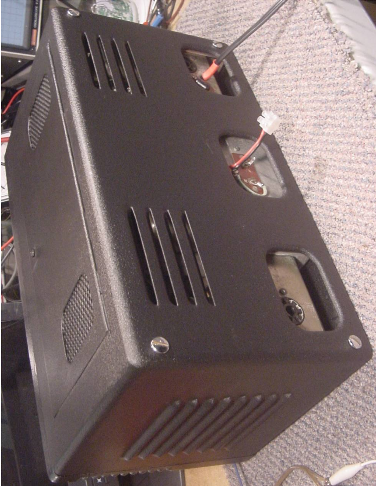
Above: Rear view of S.750 case fitted to the S.640 – note the speaker ‘pigtail’ (here terminated in a connection block) needed to allow connection to be made to a loudspeaker
